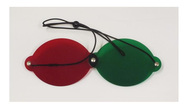
Eyeglasses for Hess examination, with red and green polarized lenses to selectively filter light spots projected on the screen.
